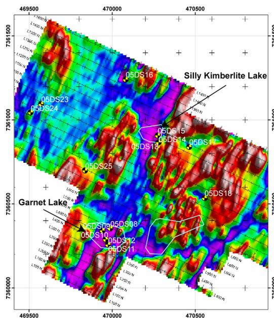
**Figure 2.** Ground based geophysical survey of the Garnet Lake area – total field. UTM coordinate system is based on WGS84 Zone 22N. Drill site locations are indicated by black/yellow circles. Note that lake shapes and locations are approximate and lie in reality ~100m W.
